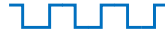
Calibration Signal Output 1kHz / 0.3V p-p Square Wave Used to Adjust Probe Equalization
